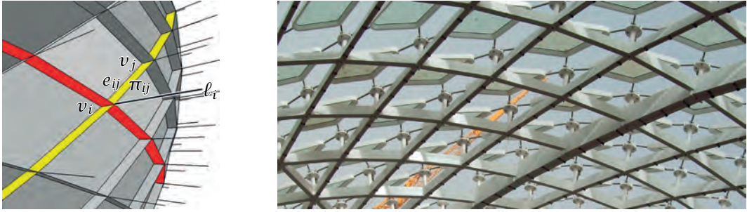
Figure 4. Torsion-free support structure. For each edge ij and vertex i of a quadrilateral mesh, we have a plane \pi_{ij} and a line \ell_i such that e_{ij}, \ell_i, \ell_j are contained in \pi_{ij} (at left, image courtesy Evolute). This support structure guides members and nodes in the outer hull of the Yas Marina hotel in Abu Dhabi, so that members have a nice intersection in each node (at right, image courtesy Waagner-Biro Stahlbau).
